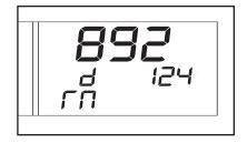
treadmill is displayed in a store. When the console is in the demo mode, the power cord can be plugged in, the key can be removed from the console, and the indicators in the display will automatically appear in a preset sequence; the buttons on the console will not operate. If a "d" appears when the information mode is selected, press the Speed – button so "d" disappears.
